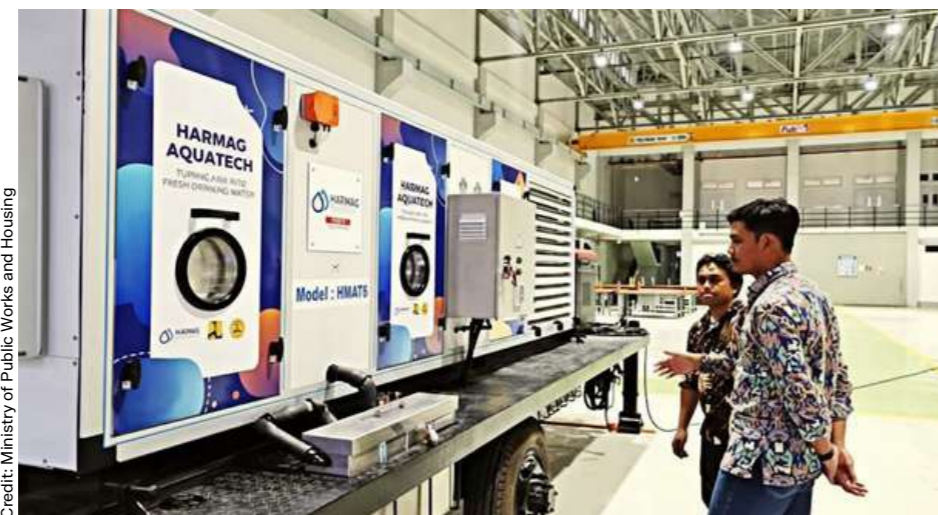
Commissioning test of the dew-water treatment technology prior to operational deployment.
